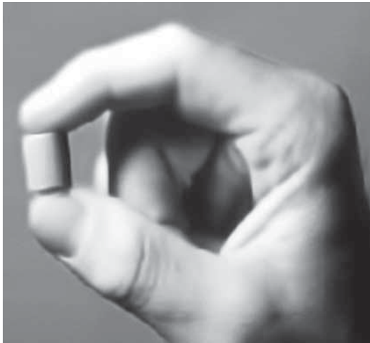
Fig. 2.1. A uranium fuel pellet.
