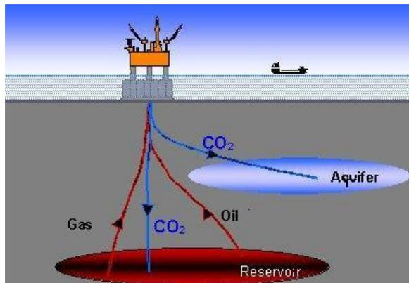
FIGURE 3. AQUIFER STORAGE AND CO<sub>2</sub> USED FOR EOR.
