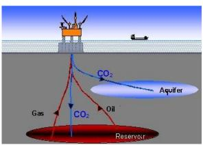
FIGURE 3. AQUIFER STORAGE AND CO2 USED FOR EOR.
